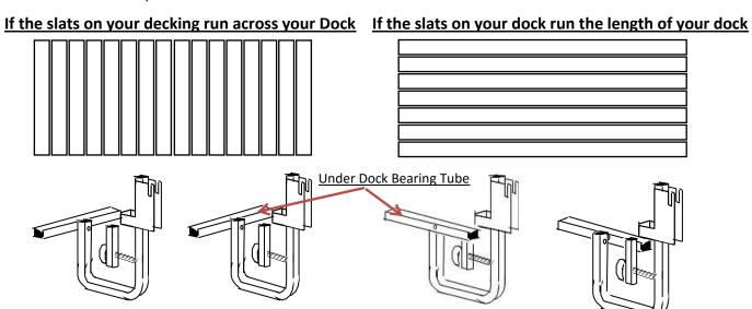
Align the under dock bearing tube as shown Align the under dock bearing tube on each side of the mount To align, undo the wing nut, remove the screw, and then align accordingly and insert the screw and tighten
